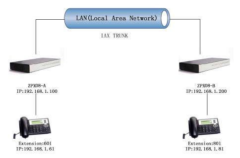
The method of connecting two ZPX08 in different location is:
