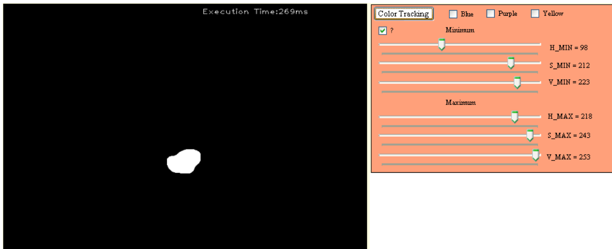
Figure 6-22 Checking the result of the automated color range adjustment after the light condition changing
