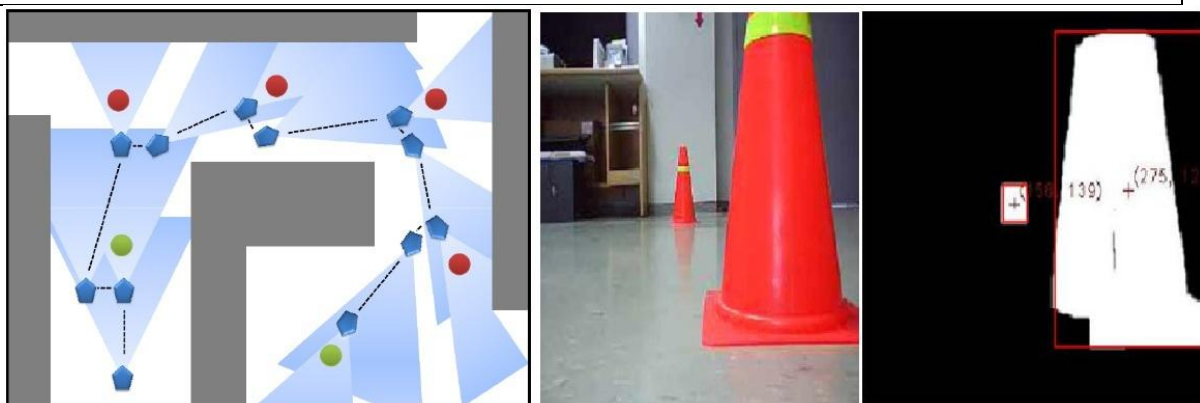
Figure 2-5 Navigation scenario and execution of the vision algorithm displaying the mass centre of the detected cone in the binary image (Begum, et al., 2010).
