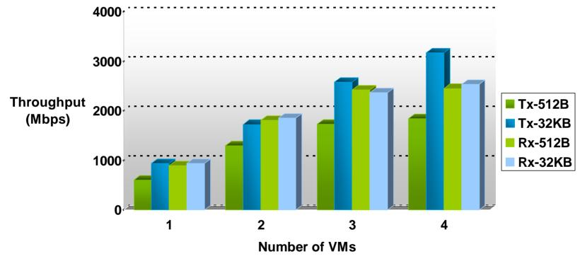
H/W:AMD Opteron 270, dual core, 2 socket, 1.99 GHz, Intel e1000 NICs S/W: ESX 3.0.1
