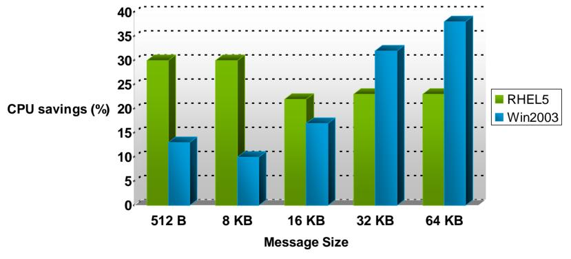
H/W: 4-way Xeon @ 3.0 GHz, Intel 82571 NIC. S/W: Virtual device: vmxnet. Netperf socket size = 64 KB.
