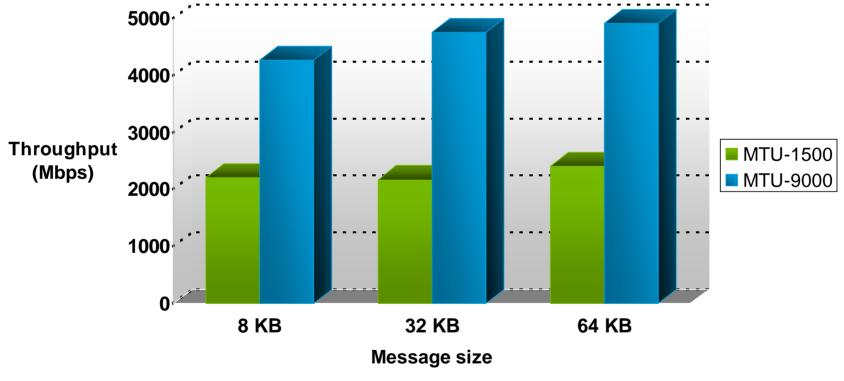
H/W: 4-way Xeon @ 3.0 GHz, Neterion PCI-X 10GigE NIC. S/W: Win 2003 64-bit. Netperf socket size = 300KB.
