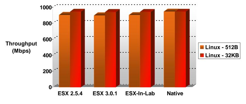
H/W: Intel Xeon 5150 Quad Core @ 2.66 GHz, Intel e1000 NIC
