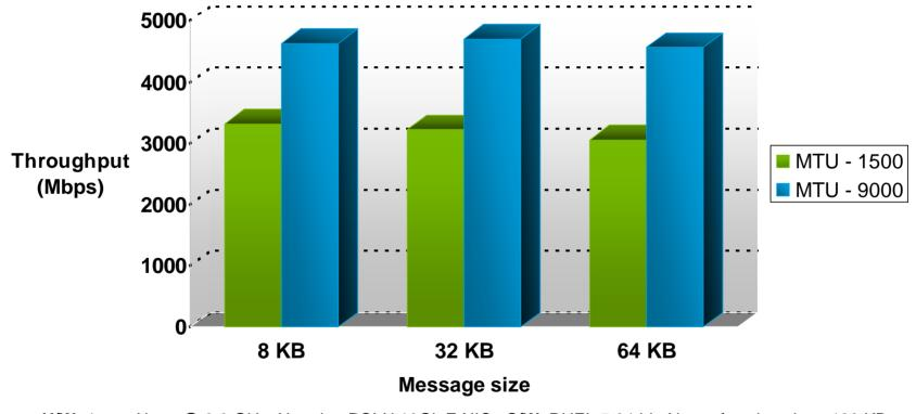
H/W: 4-way Xeon @ 3.0 GHz, Neterion PCI-X 10GigE NIC. S/W: RHEL 5 64-bit. Netperf socket size =128 KB
