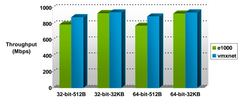
H/W: Intel Xeon 5150 Quad Core @ 2.66 GHz, Intel e1000 NIC, VT enabled for 64-bit guest, S/W: ESX in lab
