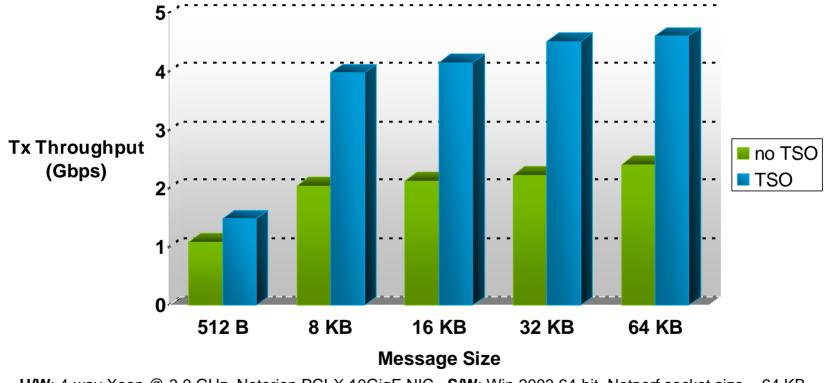
H/W: 4-way Xeon @ 3.0 GHz, Neterion PCI-X 10GigE NIC. S/W: Win 2003 64-bit. Netperf socket size = 64 KB.
