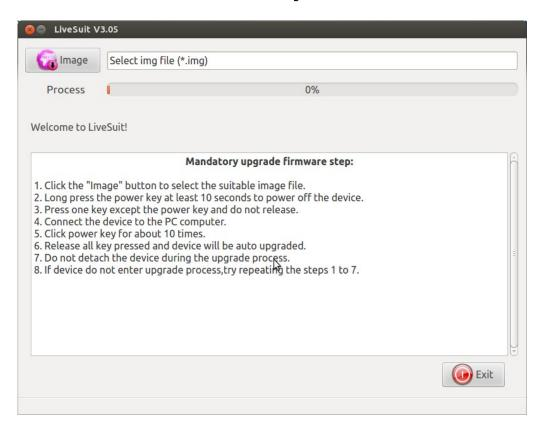
5.Closing the program or disconnecting the device When you burning firmware will break the device.
