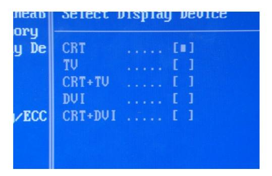
If the screen color is incorrect when using component-video out, re-enter into BIOS to select TV\_Connector in Advanced Chipset Features
