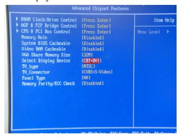
Make selections depending on different output needs: DVI Select DVI to fit DVI format CRT Select VGA to fit CRT format TV Select TV to fit Component-Video, AV, S-Video formats
