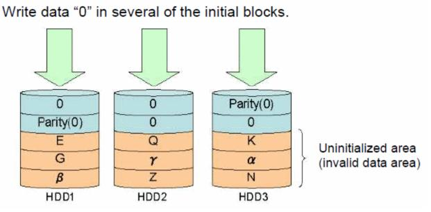
In fast initialization, zero data is written only in the top sections of the HDD units that form the disk array. The OS install information and partition information can be cleared. Since shorter processing than normal initialization is required, processing can be advanced to the next task quickly. However, as some areas are not initialized, consistency of all the disk array areas is not established.
