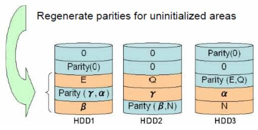
When fast initialization is executed, normal initialization is interrupted, or initialization is not executed for the disk array, the disk array contains uninitialized areas. Background initialization is the function that matches the parities for all the uninitialized areas in background.
