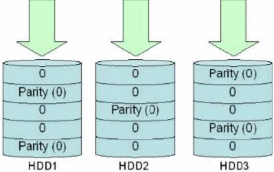
In normal initialization, zero data is written to all the HDD areas that configure the disk array. Since the information in the HDD is cleared to 0, the entire invalid data that has been originally stored in the HDD can be deleted. Since all zero data is recorded, the consistency of the parity information is also restored.
