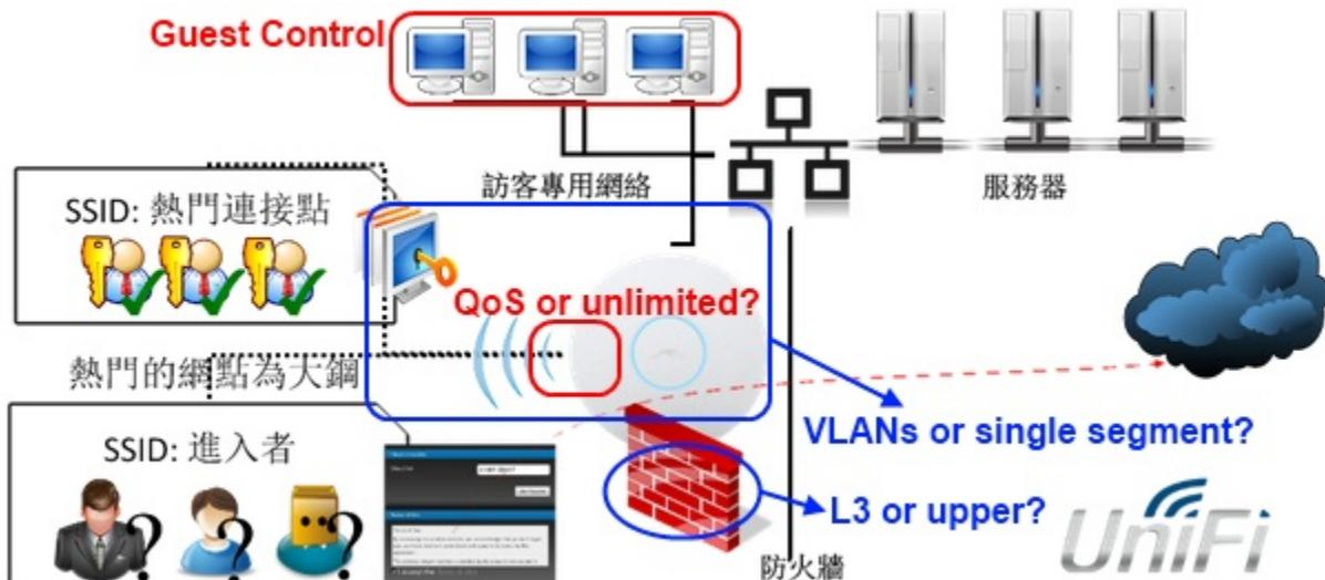
UniFi AP solution????????????????????(Guest Control), ??????????, ??????????????QoS????(Traffic Shaping), ?????????????BYOD??, ??????????. ???SSID?????????????, ???VLAN????????????????, ??????. ???AP??????????, ?????????????????(Controller)??????????.
