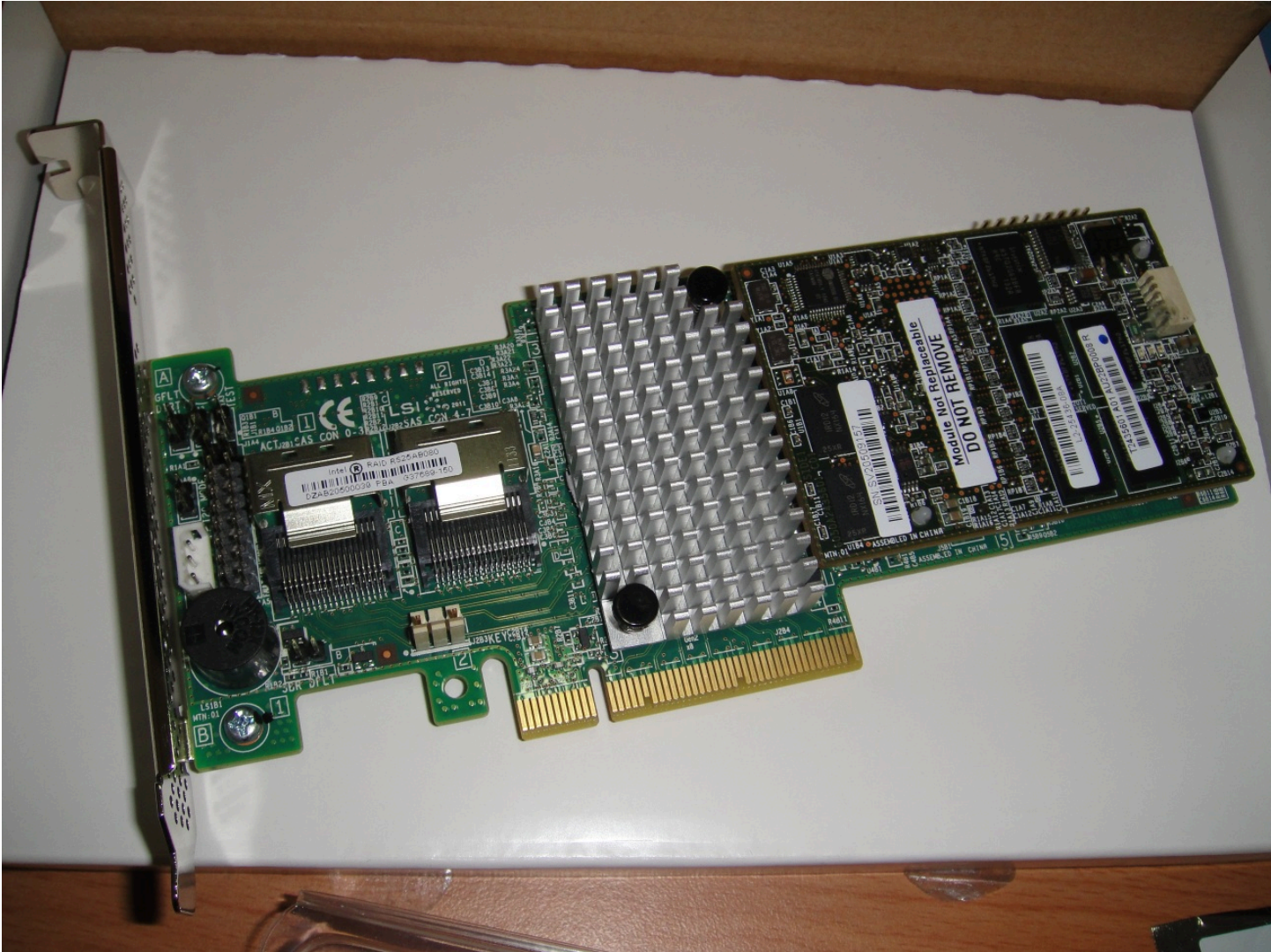
Low profile, ??????2U?????. ?????????????????, ??????????LSISAS2208 RoC ASIC chip.
